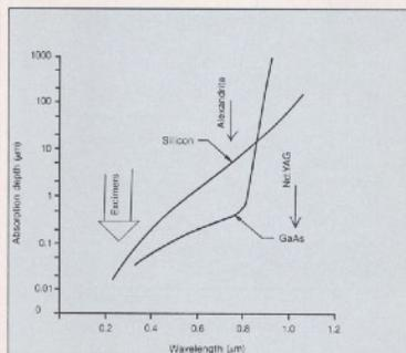
Figure 1. Absorption depth of silicon and gallium arsenide as a function of wavelength, with common laser wavelengths noted.
